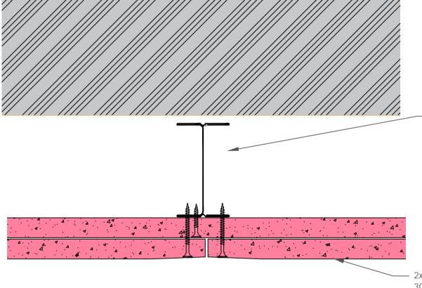
SPEEDLINE 70mm 'I' Studs at 600mm Ctrs
